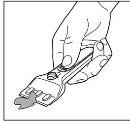
1. Slide back the upper part to render the inserted blade visible. If the screw is too loose or too tight, adjust it accordingly with a screwdriver.
